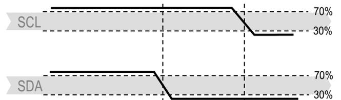
Figure 18 Start Transmit State (S) - When SCL is at high level, SDA is converted from high level to low level. The start state is a special bus state controlled by the main engine, indicating the start of slave machine transit (after Start, BUS is generally considered to be in a busy state).
