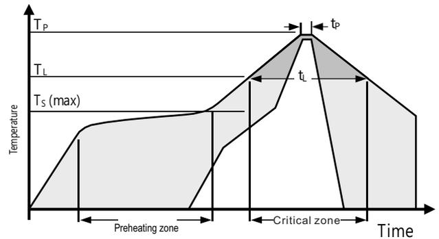
Figure 9 JEDEC Standard welding procedure diagram.  $T_p \leq 260^\circ\text{C}$ ,  $t_p < 30$  sec, lead-free welding.  $T_L < 220^\circ\text{C}$ ,  $t_t < 150$  sec, The rate of temperature rise and fall during welding shall be  $< 5^\circ\text{C}/\text{sec}$ .
