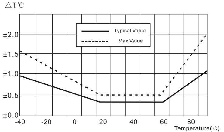
Figure 3 Typical error and maximum error of temperature
